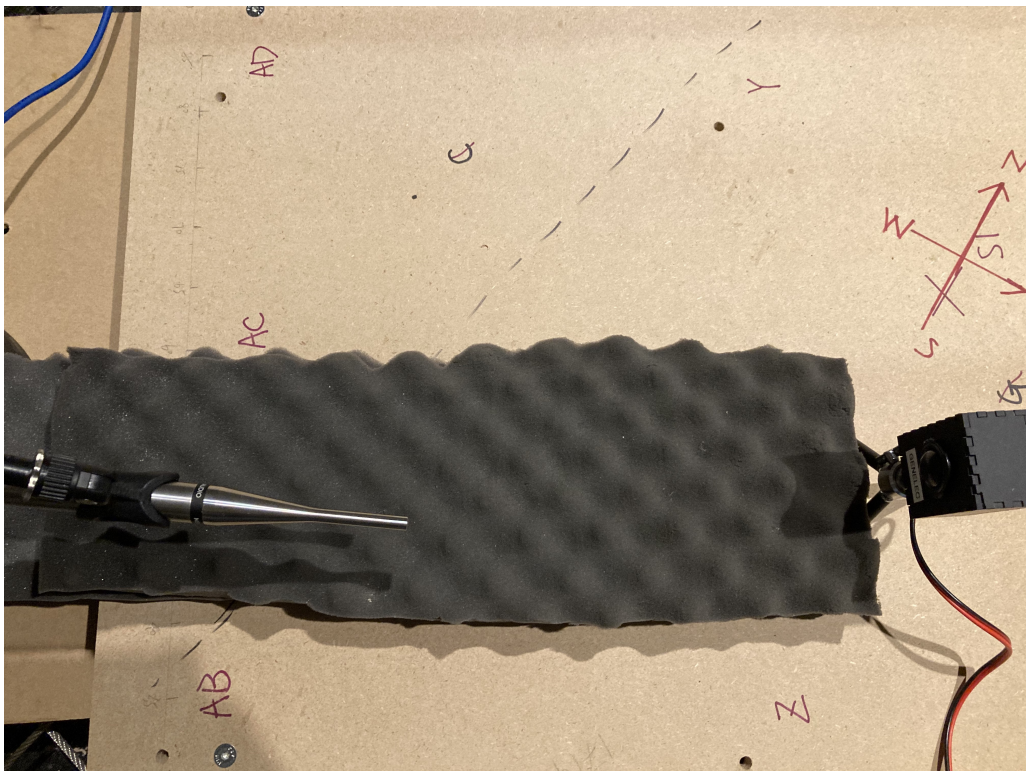
FIGURE A.43: A picture of tweeter response measurement. The M30 microphone was tilted slightly right to capture the responses.
