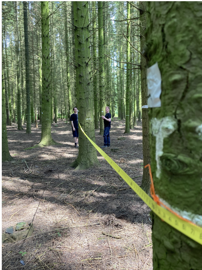
FIGURE A.14: The measurement of the tree has no clear sight to the standing point was noted with a soft measure tape.
