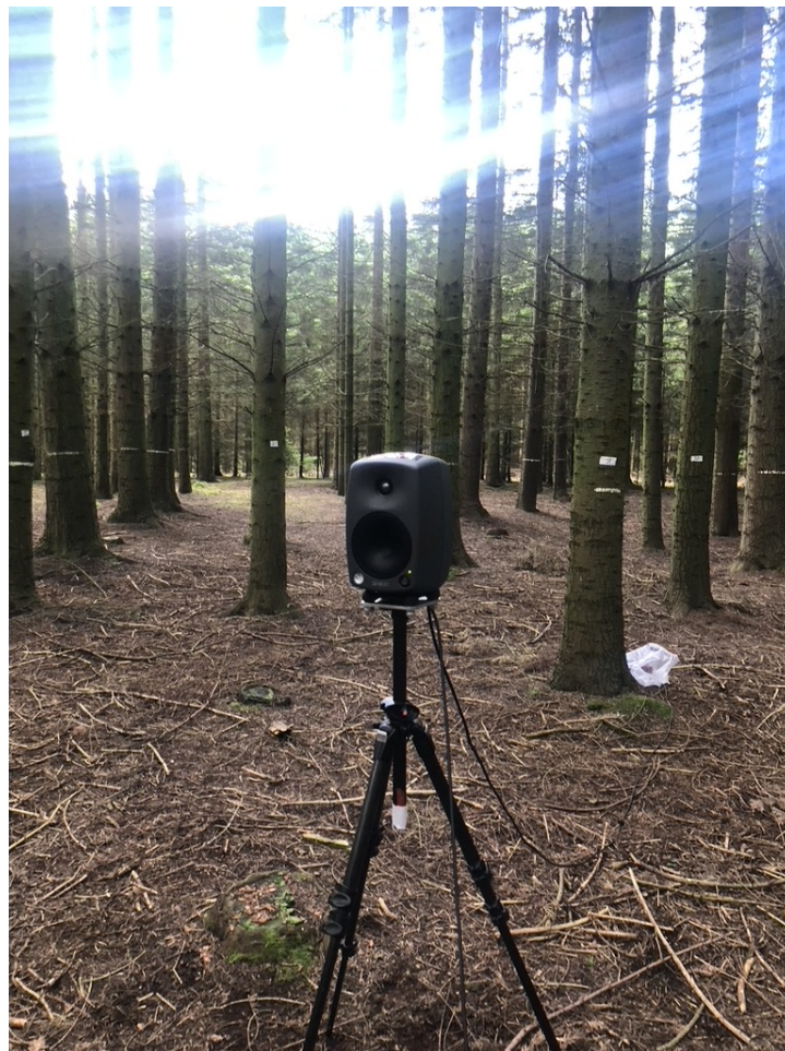
FIGURE A.8: A Geenelec 8130A loudspeaker was used as the source at the height of 1.5 m for the forest IR measurement. The speaker was powered by an inverter generator placed on the ground and covered in a plastic bag.
