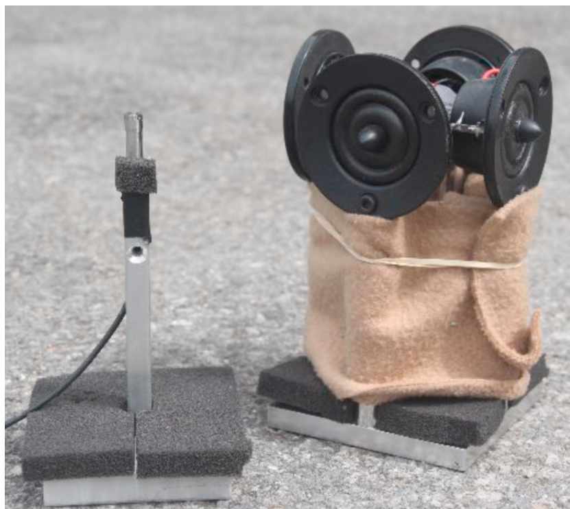
FIGURE A.5: The microphone (left) and loudspeakers array (right) used in Stonehenge scale model. From [9].
