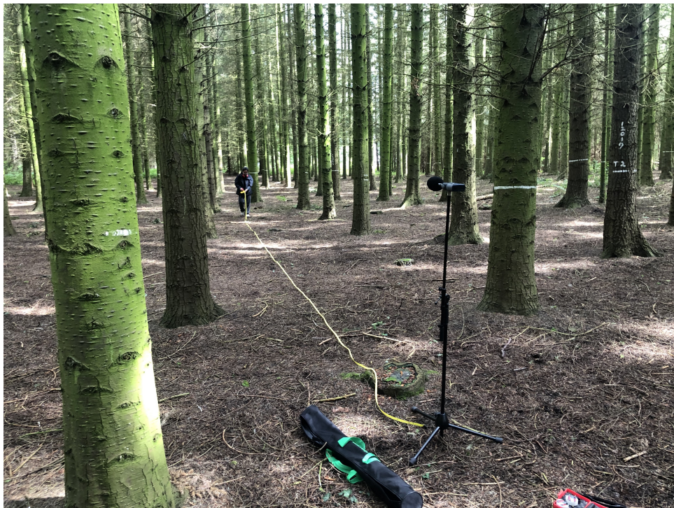
FIGURE A.21: Measure sound attenuation in the same forest environment as the IR measurement. The receiver position was not moved during the measurement, and the source position was found using a tape measure.
