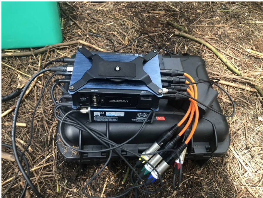
(B) The recorders connections. Four breakout leads were used to reduce the gain from the Soundfield recorder to the Zoom recorder.
