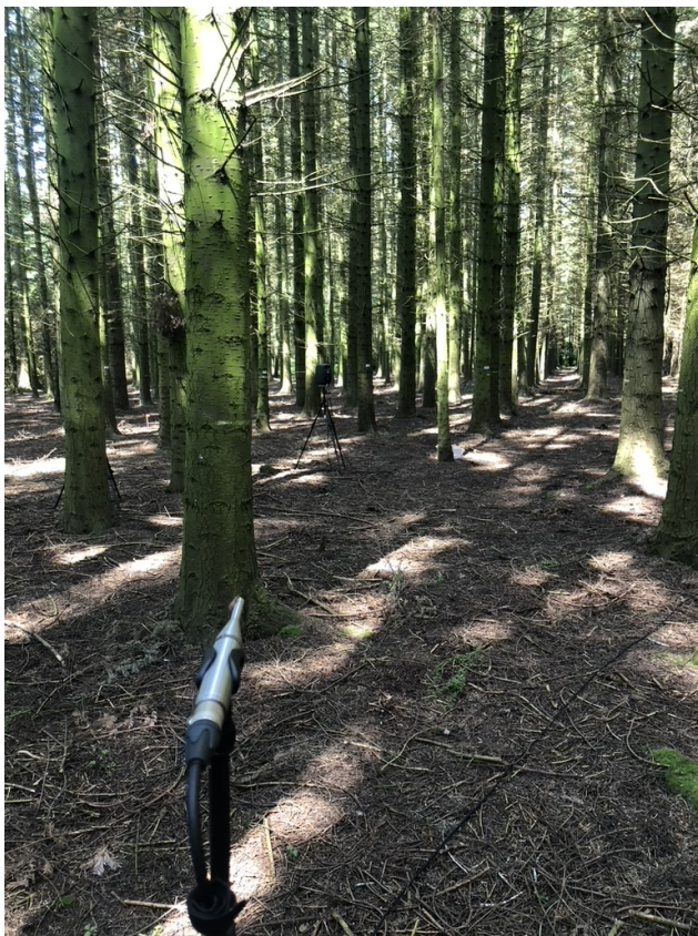
(A) An Earthworks M30 measurement microphone placed at the height of 1.5 m.
