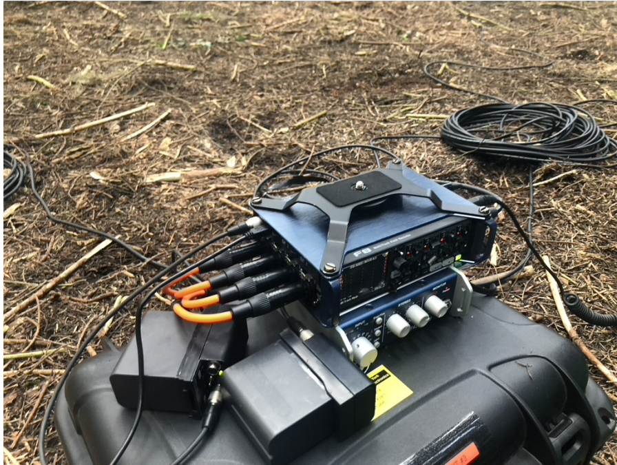
(A) A Soundfield ST450 MkII recorder (bottom) and a Zoom F8 multitrack field recorder (top) were powered by two Sony battery packs separately.
