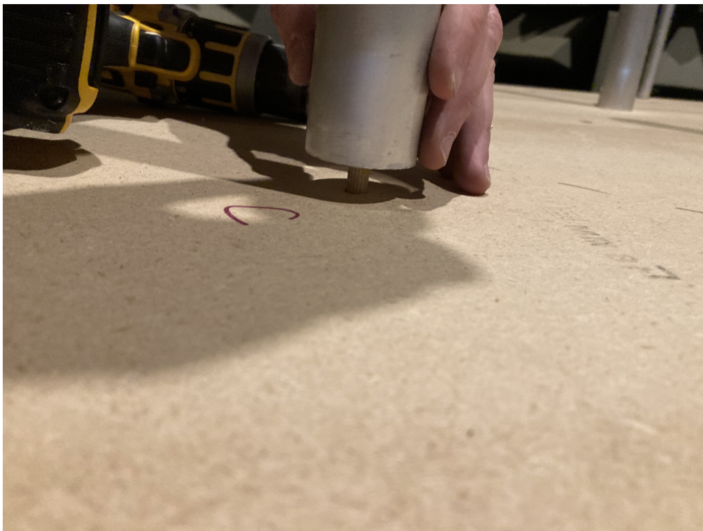
FIGURE A.35: A picture of the modelled tree trunk doweling in the board.
