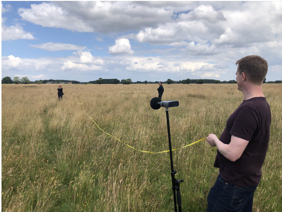
FIGURE A.20: Measure sound attenuation in an open field in Heslington Tillmire Site. The source used was a stater pistol and the receiver was a sound level meter. The measurement height was 1.5 m.
