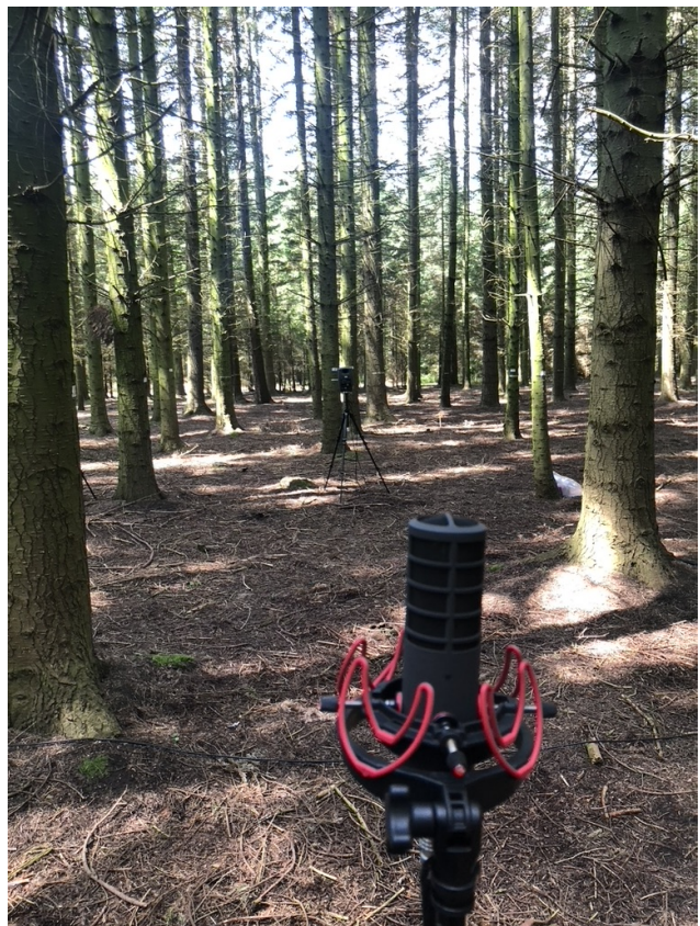
(B) A Soundfield ST450 MkII microphone placed at the height of 1.5 m.
