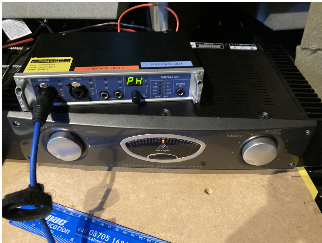
FIGURE A.38: A Reference Amplifier A500 preamp (bottom) and a Fireface UCX interface (top) were used in the scale model measurement.
