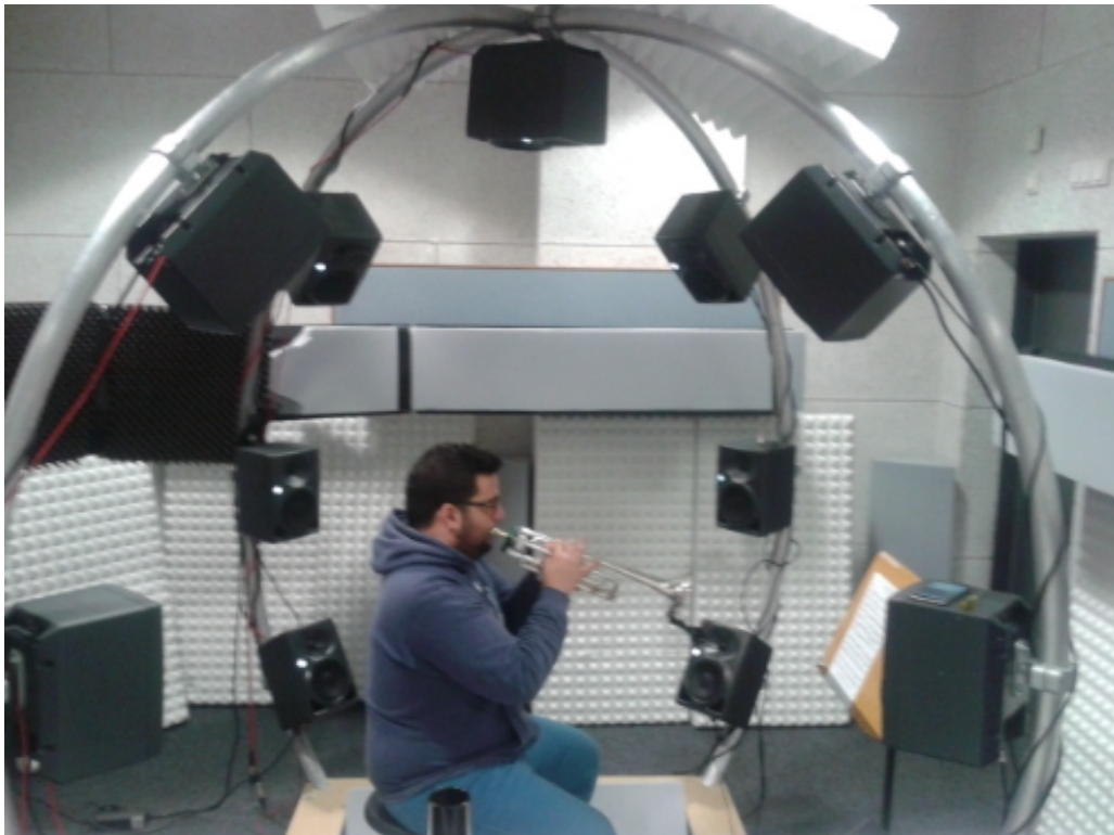
FIGURE 2.4: A photograph of Amengual et al. (2016)'s [25] virtual acoustic simulation rig with trumpet player performing.
