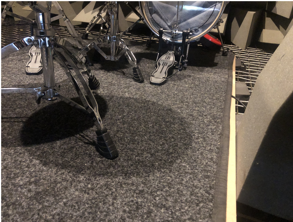
FIGURE 3.5: Drum rug used to cover the MDF board reducing slip and providing more accurate floor reflections.
