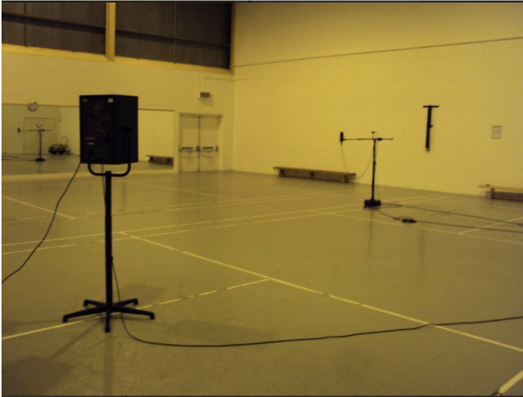
FIGURE 2.2: An RIR measurement taken at the University of York Sports Centre. Image taken from OpenAIR [4]
