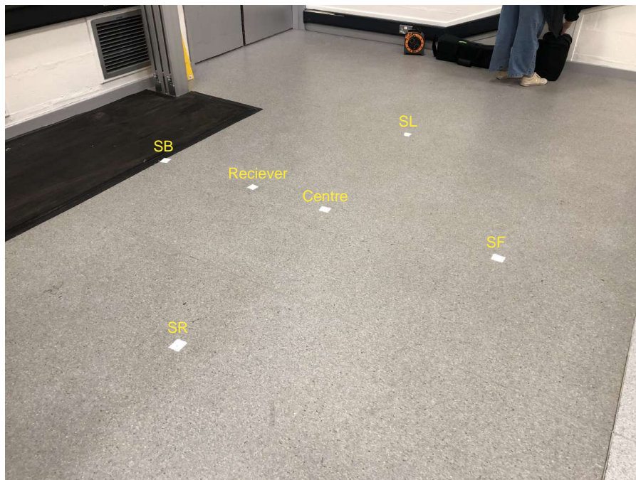
FIGURE 3.21: Floor markings of source, receiver & centre positions for SRIR measurements in PL001.
