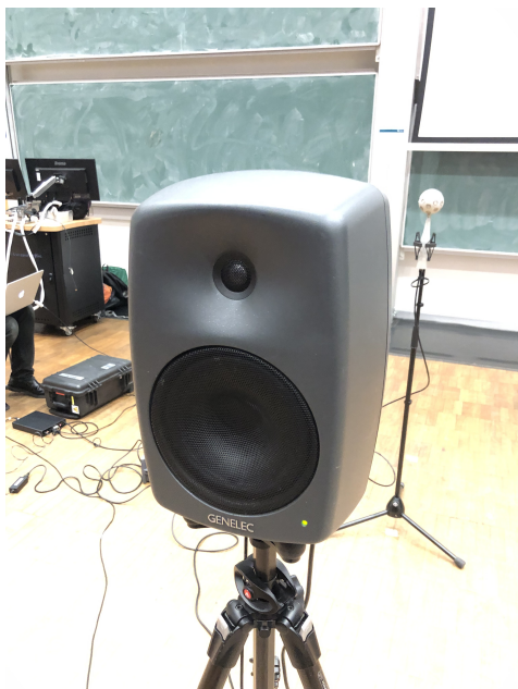
(A) Source used in SRIR measurement- Genelec 8040A
