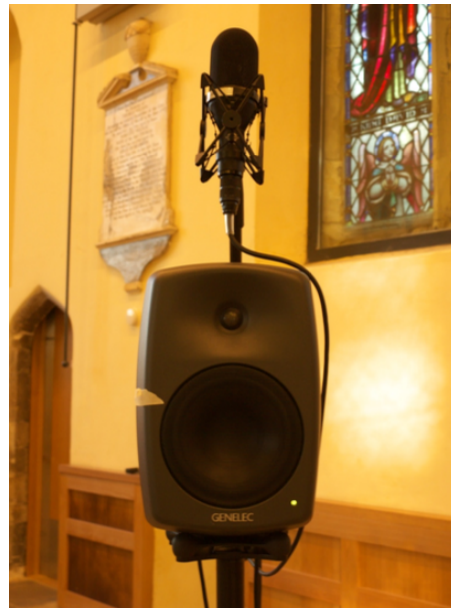
FIGURE 2.10: “Position of Soundfield Microphone placed above the Genelec 8040 loudspeaker used to measure performer position SRIRs in the real performance space” From [19]
