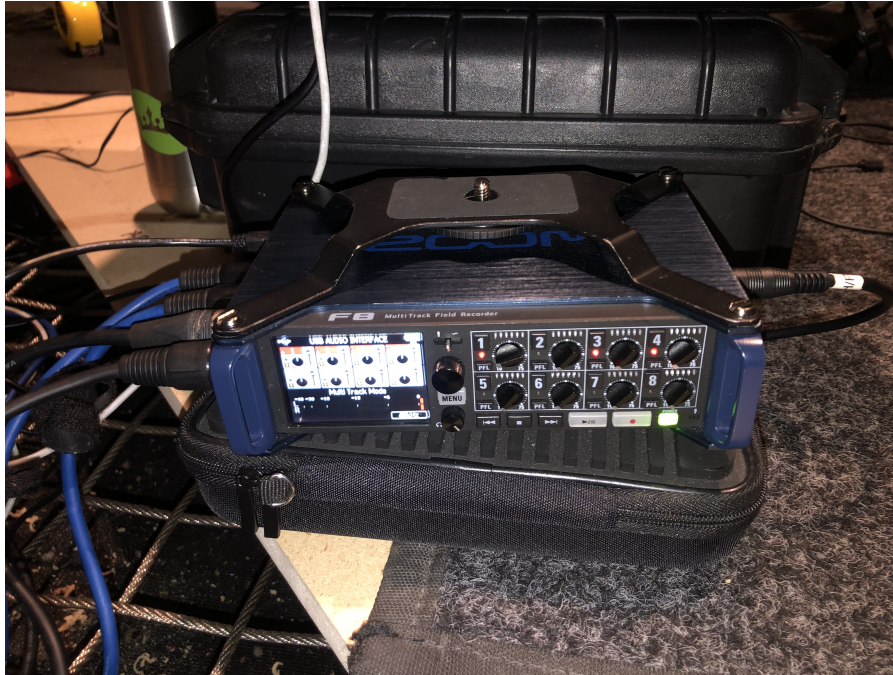
FIGURE 3.14: An image of the Zoom F8 multitrack field recorder used in the final build of the VDR.
