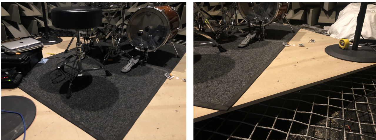
FIGURE 3.30: Images of the MDF platform the drum kit was situated on in the anechoic chamber.
