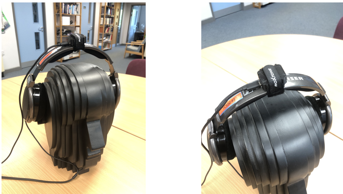
FIGURE 3.27: Images of the NV Sonic head tracker attached to a pair of headphones and worn by a model head.
