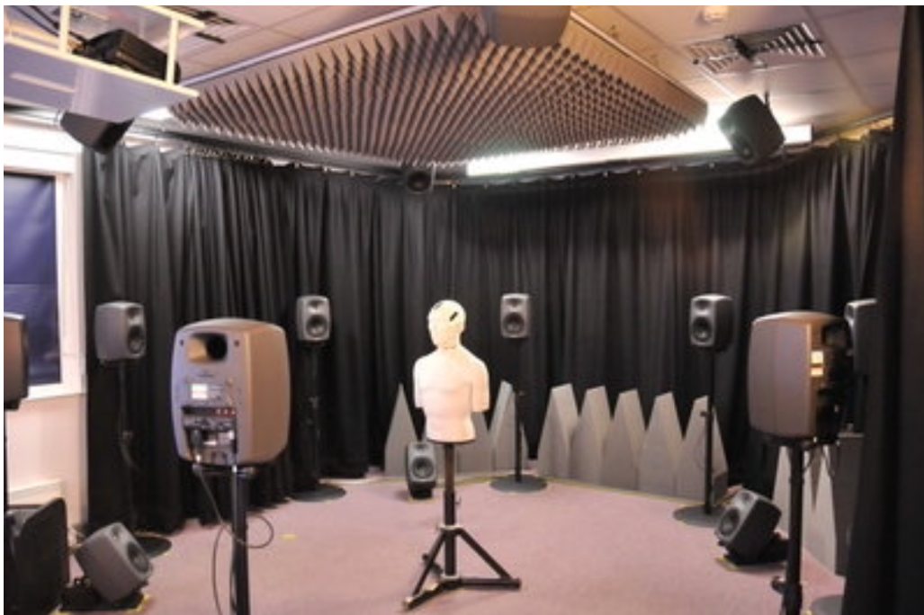
FIGURE 2.5: “ Photograph of the Virtual Singing Studio as set up in the acoustically treated listening room (KEMAR denotes position singer would take) ” [19]
